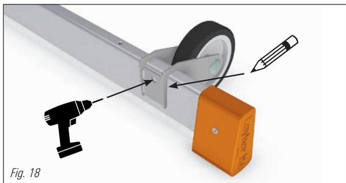
3. Rotate the cross-piece roller horizontally by 180° and align it on the mark, and also drill through the hole in the mounting.
