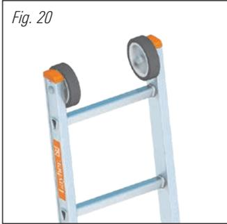
For easier and more ergonomic use of long extension ladders and all-purpose ladders, they can be retrofitted with top rollers. To do so, a through-hole must be drilled as shown in the drawing excerpt.
